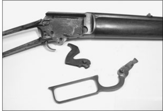
Shown here with the hammer, lever, and carrier removed, the action is nearly bare. And all this took barely a few seconds to accomplish.
