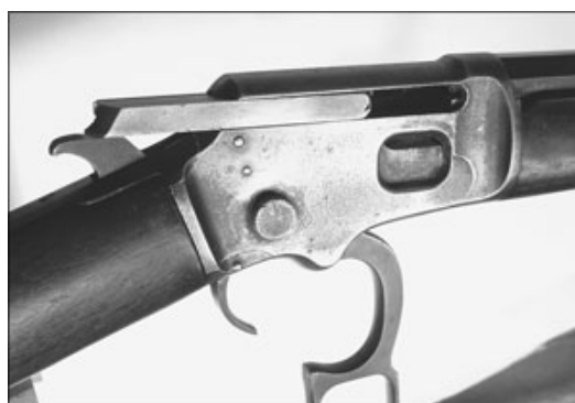
The 1891 Marlin is shown here with its action open. This is where you look to be sure the rifle is empty before you start in with any work.
